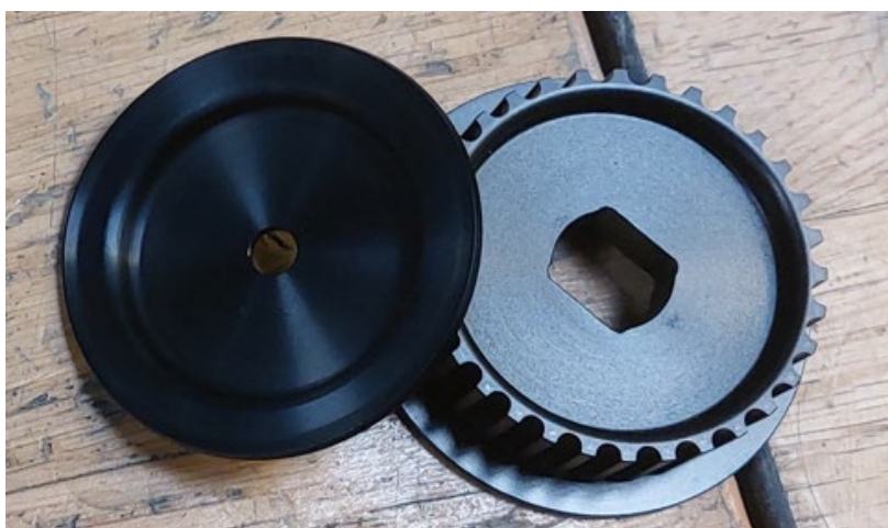
Figure 2: Rear pulley with flange 547028401 + 546080601.
