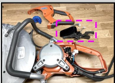
5 Mount the display and connect the three cable connectors.
