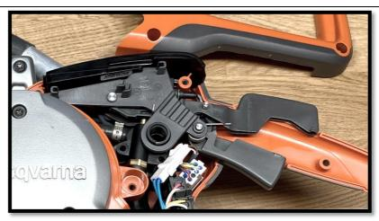
Reattach the blue valve, add the cover and screw the 8 screws back in (2,5Nm).
