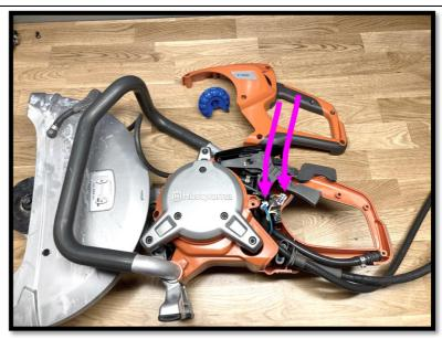
4 Lift out and replace the trigger console and display.
