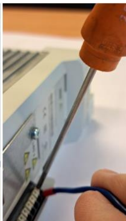
Pull out wire while pushing
