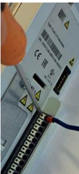
Push in connector with a screwdriver
