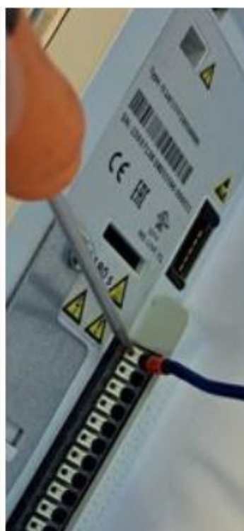
Push in connector with a screwdriver
