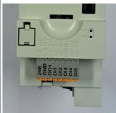
I550 has a detachable connector with connections at both sides
