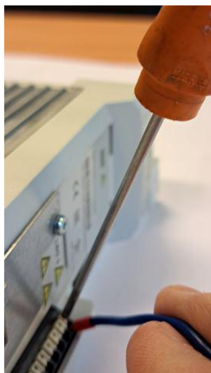
Pull out wire while pushing
