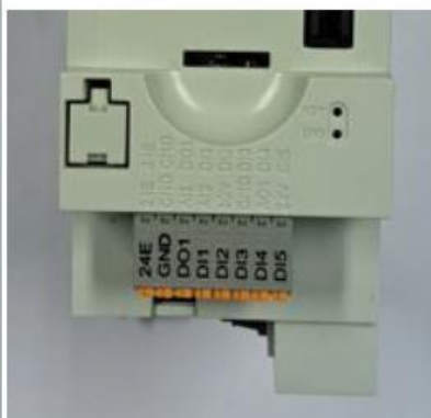
I550 has a detachable connector with connections at both side
