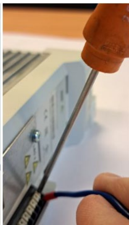
Pull out wire while pushing
