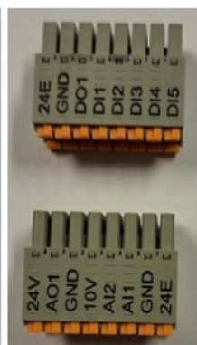
I550 has a detachable connector with connections at both side
