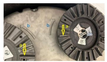
Note: This reprogramming is only needed if the 4 discs rotate in the wrong direction (a) compared to the arrows (b).
