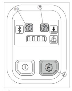
2. Toggle between e-gear modes by short-pressing the gear button E(A).
