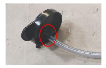
• Change the hydraulic oil cooler fan fuse. Use 535612501 from the upgrade kit 546006801.
