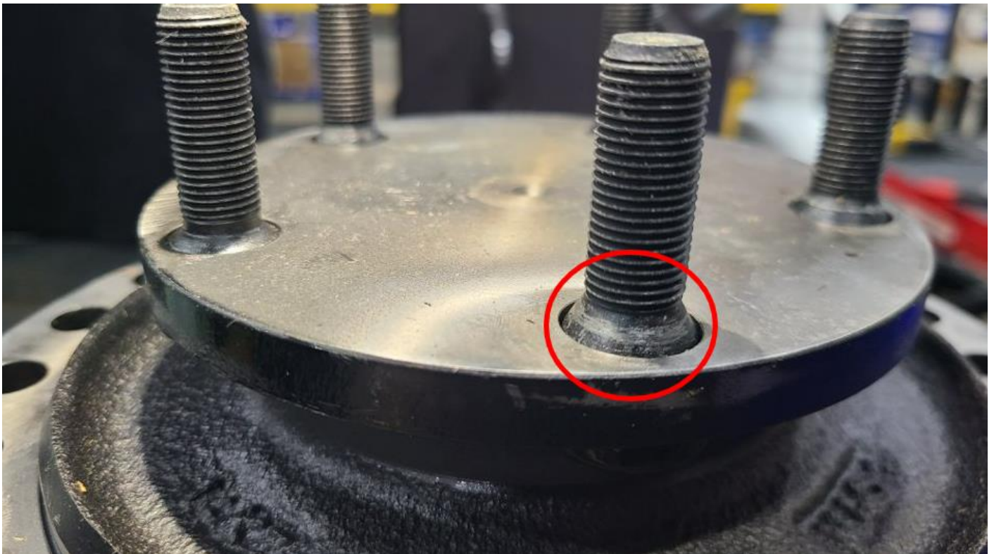
Fig. 1: New type of motor flange stud with increased chamfer.
