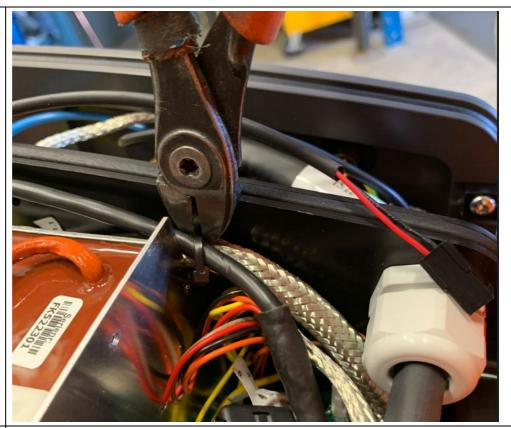
8 Use 2 cable ties to clamp fan cable and FKD cable to the fan bracket.
