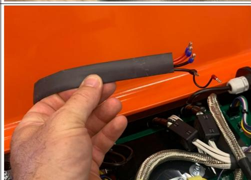
16 Flip the PP around and pull out the cable.
