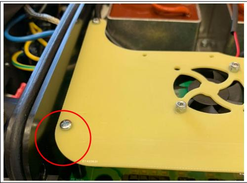
Reuse the long screws that was diassambled in step 2 to assemble the fan on the FKD board.
