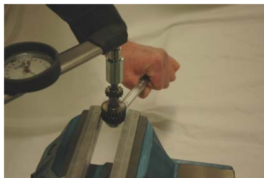
If the torque is higher, you need to adjust to the correct figure.
