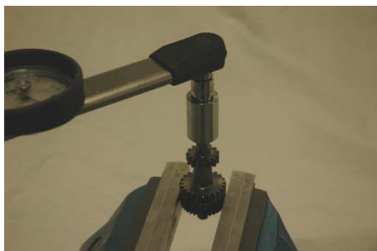
Check the torque. If it less then 17 Nm (15 Nm USA), replace the Kit Wear Parts.
