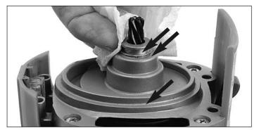
Carefully clean around the O-rings and the surface touching gasket 510 44 09-01 in the cover.
