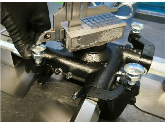
2. Press and hold the blade arm shoulder to remove the clearances. Adjust the screws to be on equal height.
