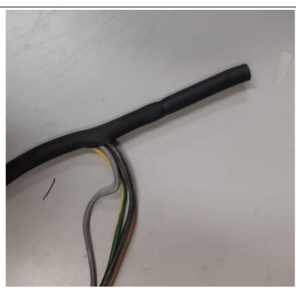
Move the cable markings from the cut part to the cable. Attach cable sleeves.
