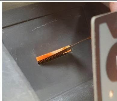
Align the HMI panel with the designated area on the outer cover and press down.
