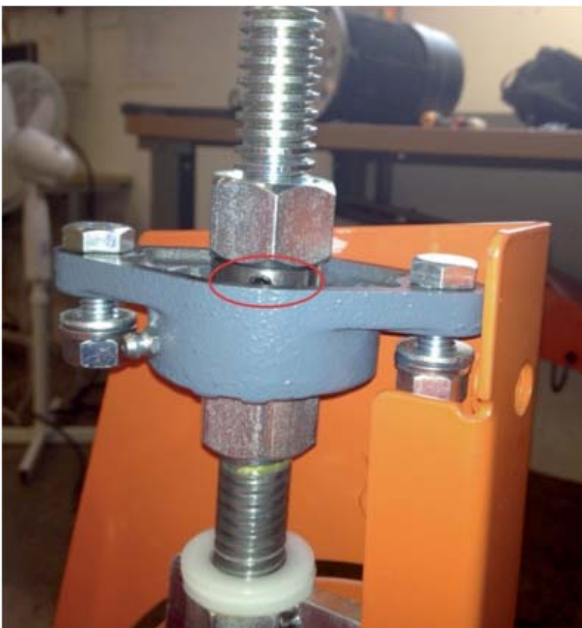
Picture 2 The SKF bearing correct mounted on the machine.
