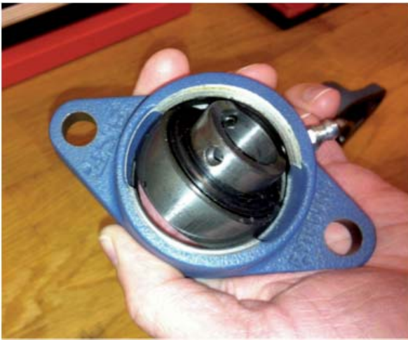
Picture 1 Rotate the inner part of the bearing 180°
