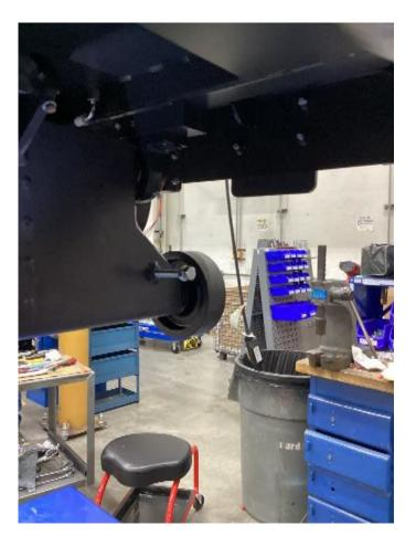
Reinstall side panels. Lift saw and return depth stop bolts to proper height for blade.
