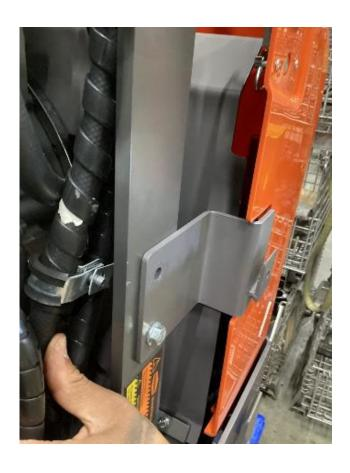
Remove top nut and bolt from right upper blade guard spade holding fuel hose clamp.
