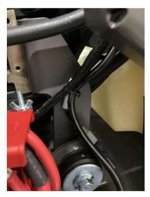
Reconnect HMI Cable to Cowl. Replace zip tie holding cables to Left Engine mount. Trim off zip tie tails.
