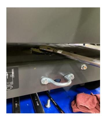
Nut and washer must be cleaned of any Loctite residue. Clean or replace nut to ensure new Loctite will perform as expected. Once the parts are clean reapply Loctite 263 to threads on nut. Just enough to coat the grooves of the threads. Tighten nut with wrench then Torque to 280 Nm.
