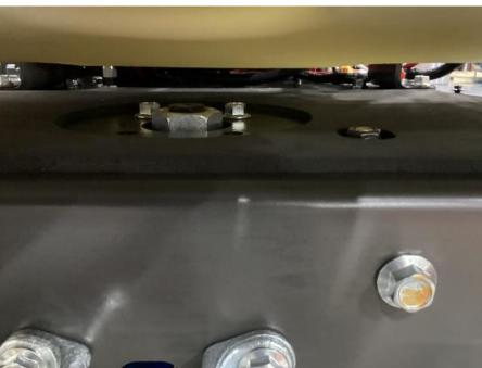
Remove back two flange bolts from baseplate to axle. (16mm Combination Wrench or 16mm Socket and 3/8' Drive Ratchet)
