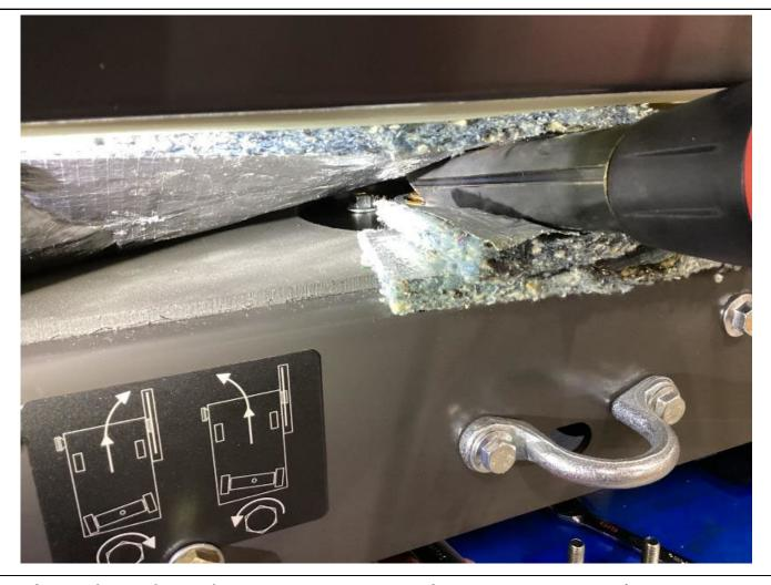
Use an insulated pad and an extension tube to position heat gun over nut. Heat nut to a minimum 120°C/250 Fahrenheit to release Loctite from nut. Be very cautious and protect fuel tank and insulator pad from heat. (Heat gun with Ext tube, Infrared Thermometer)
