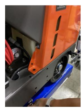
With Cowl secured from overhead. Remove the bolt from rear lift bail bracket connected to cowl. Then remove 4 bolts holding the cowl to the baseplate.
