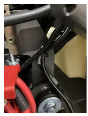
Disconnect HMI Cable to Cowl. Remove zip tie holding hose near the cables on the Left Engine mount.
