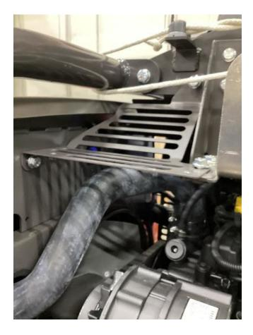
Lower Cowl back down onto baseplate. Install 4 bolts back into baseplate, then reattach Lift bail to cowl bracket. Torque Lift bail bolt to 50 Nm. Torque The 4 cowl bolts to 81 Nm.
