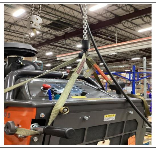
Secure Cowl with overhead hoist. Saw should be sitting stable on all four wheels and a 4 x 4 block or equivalent under front as shown on page 4.
