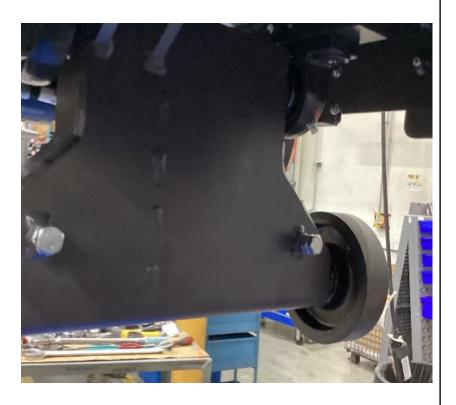
With Saw securely raised or lifted, loosen jam nuts and lower depth adjustment bolts all the way down.
