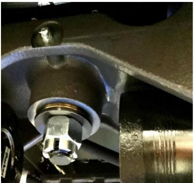
Lift saw securely to prevent falling or dropping. Once saw is secure, access area under rear axle to remove cotter pin from castle nut. Then loosen nut about two turns.
