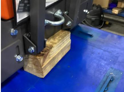
Lower saw on work area so all the wheels are on the ground or table. Place a block under the frame in front of the blade shaft. This will help to prevent saw from tipping when cowl is removed.
