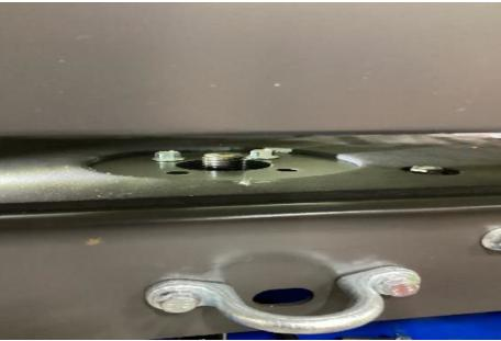
If nut is loose already, inspect parts for damage or wear. Replace any parts that are suspect.
