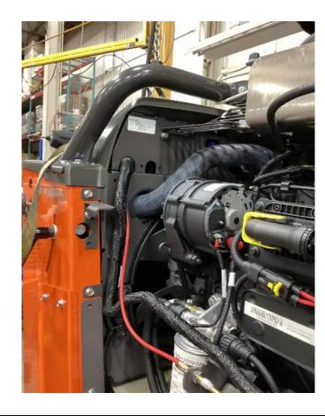
Remove protection brackets from right side of saw.
