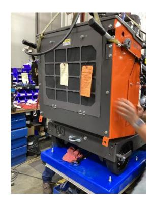
Carefully lift cowl up and back slightly about 3-4" from baseplate.
