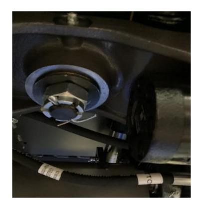
Tighten lower nut on rear axle. Nut should turn at least a ¼ turn after contact but no more than half a turn. Line up hole in shaft with slots in castle nut to secure with cotter pin. Insert cotter pin and bend as shown.
