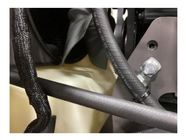
As you lift, watch fan blade and position blades like shown to get maximum clearance from fuel tank. Do not stretch hoses and cables too far.
