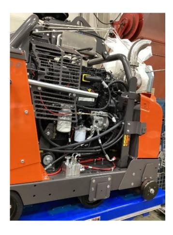
Remove Side panels from both sides of saw. (Flat Head Screwdriver)
