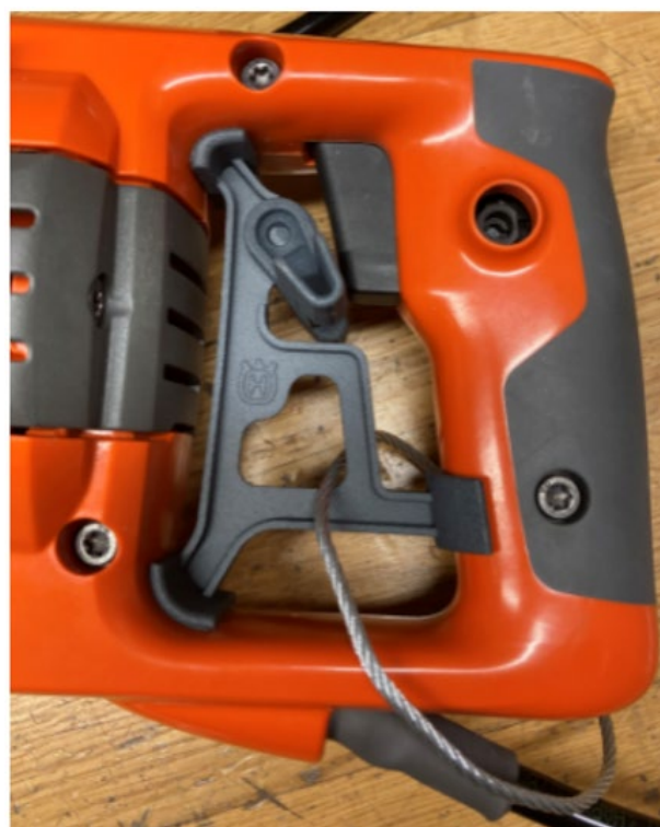
Figure 1: New Trigger-Lock Bracket installed.
