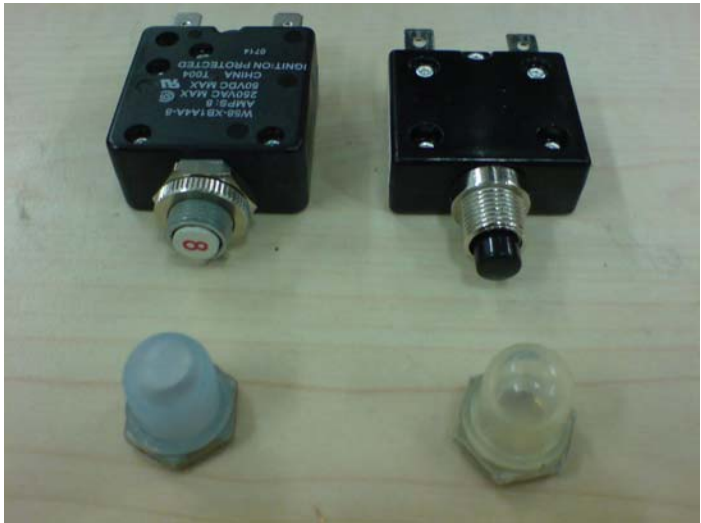
Picture 3. The new circuit breaker is shown to the left and old type to the right
