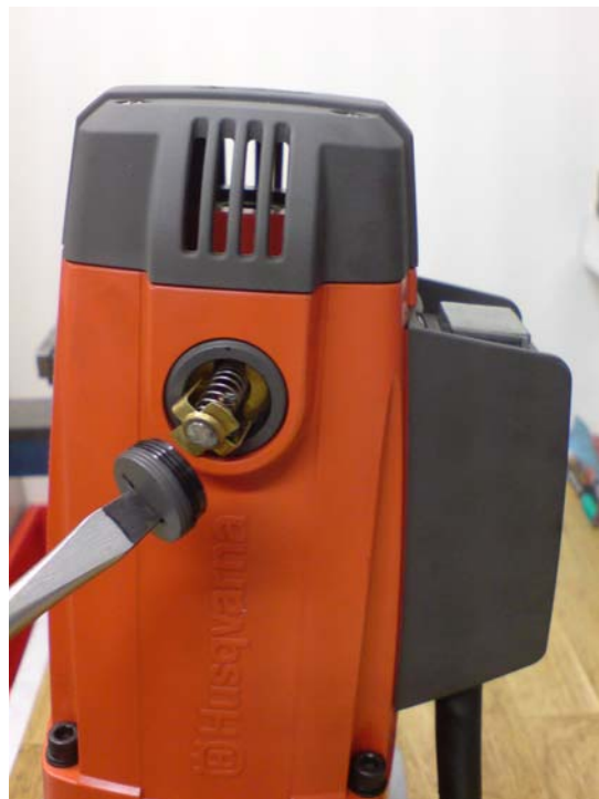
Picture 12. Reinstall brush and screw
