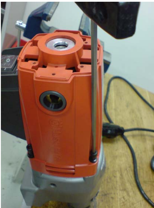
Picture 11. Tighten motor housing screws to 4Nm
