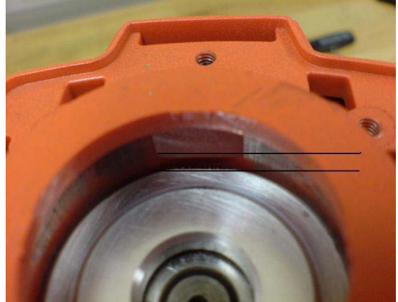
Picture 10. Planes should be parallel
