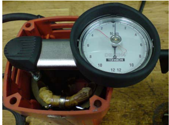
Picture 6 Tighten stator screws
