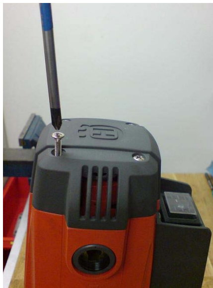
Picture 2. removing the back cap screws
