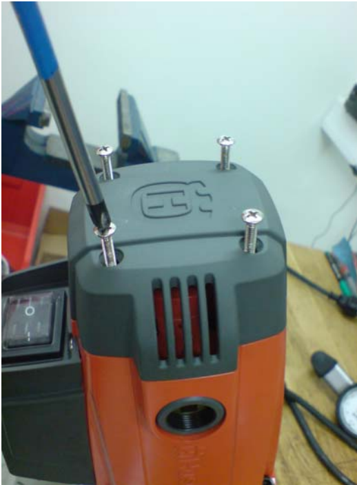
Picture 13. Reinstall back cap screws
