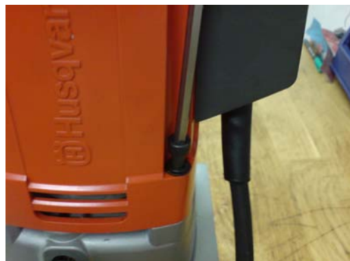
Picture 4 removal of the motor house screws
