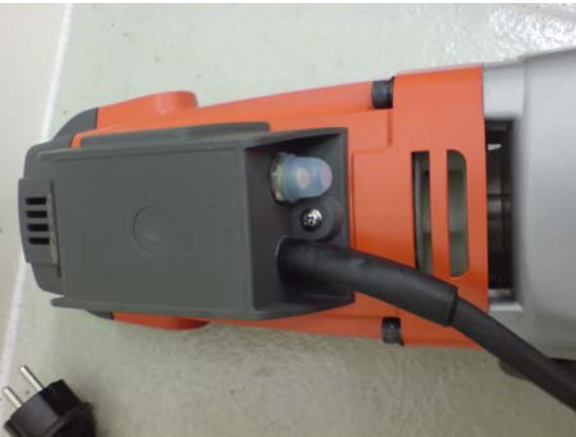
Picture 1. New type with blue silicone dust cover (522 81 11-02)
