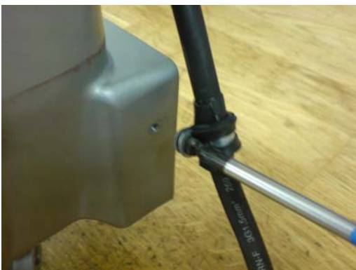
Picture 3 removal of the cable clamp
