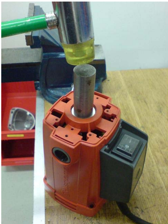
Picture 7 removal of the bearing support
