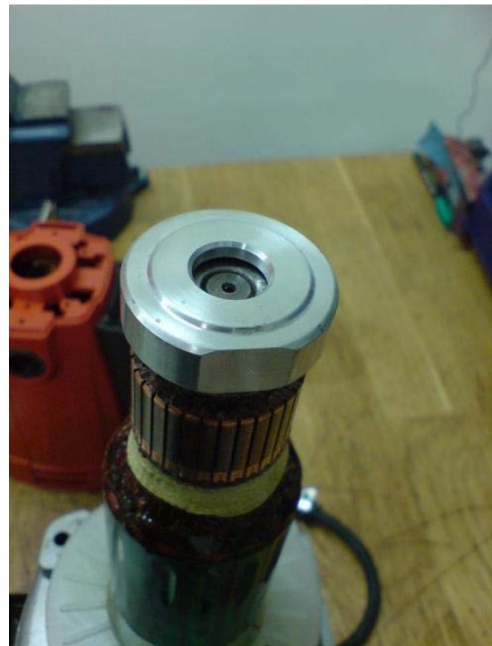
Picture 8. Assembling the bearing support
